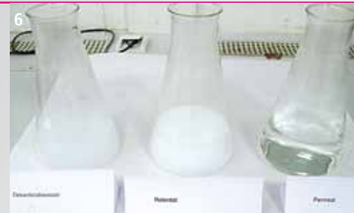
Figure 6: Efficiency of the process (left, water directly from S-PVC production; centre, retentate [concentrated]; right, filtered water)
